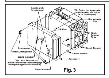
Position accessory unit against the side of the breaker carefully to determine that all accessory actuator blades are engaged into the pin slots of the circuit breaker.
