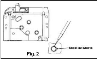
DO NOT use excessive force or the internal mechanism of the circuit breaker may be damaged.
