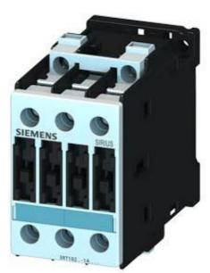
Power contactor, AC-3 25 A, 11 kW / 400 V 110 V AC, 50 Hz / 120 V, 60 Hz 3-pole, Size S0 Screw terminal !!! Phased-out product !!! Successor is SIRIUS 3RT2 Preferred successor type is >>3RT2026-1AK60<<
