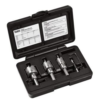
This 4-piece Carbide-Tipped Hole Cutter kit cuts quick, precise holes in a variety of materials. Set includes three commonly used sizes plus an extra pilot bit. Integrated flange prevents the operator from drilling beyond the sheet metal. Split point pilot drill bit prevents bit walking.
