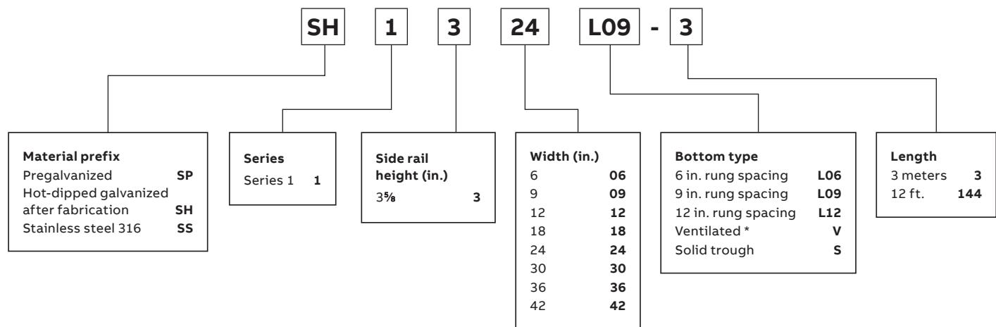
\* For load CSA class C3M, NEMA 8C or less, please see an alternative ventilated series of cable tray called One-Piece found on pages A174 to A207 of this catalogue.
