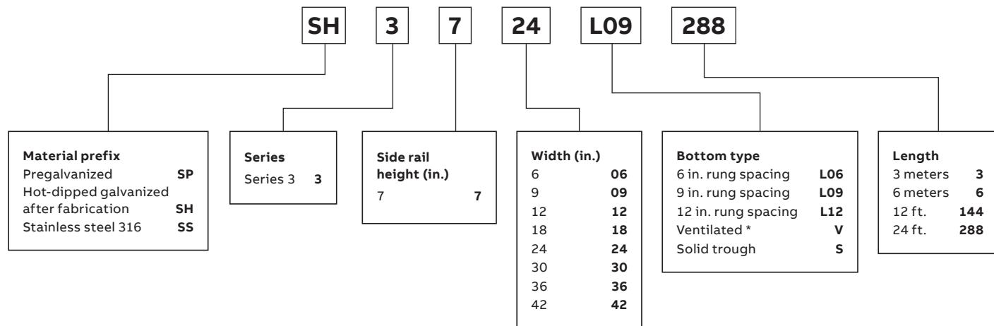
\* For load ratings of CSA class C/NEMA 12C or less, please see an alternative ventilated series of cable tray called One-Piece found on pages A174 to A207 of this catalogue.
