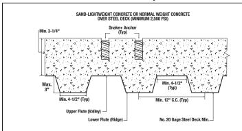
1. 3/8-inch diameter anchors may be placed in the topside of steel deck profiles provided the minimum topping thickness, minimum spacing distance and minimum edge distance are satisfied as given in the installation information table.
