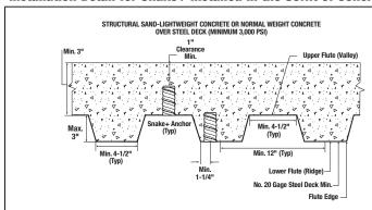
Anchors may be placed in the upper flute or lower flute of the steel deck profiles provided in minimum hole clearance is satisfied. Anchors in the lower flute may be installed with a maximum 1-inch offset in either direction from the center of the flute. The offset distance may be increased proportionally for profiles with lower flute widths greater than those shown provided the minimum lower flute edge distance is also satisfied.
