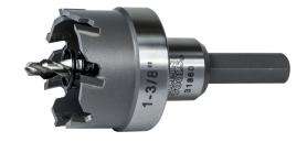
This carbide hole cutter cuts quick, precise holes in a variety of materials. Integrated flange prevents the operator from drilling beyond the sheet metal. Split point pilot drill bit prevents bit walking.
