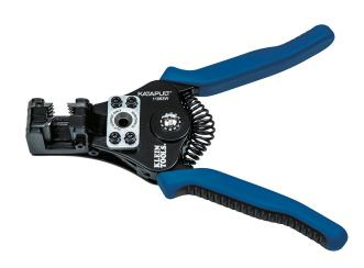
Klein Tools' Katapult® Solid and Stranded Wire Stripper / Cutter has a built-in cutting hole to cleanly cut 8-20 AWG solid and 10-22 AWG stranded wire, while the stripping head allows you to easily grip and strip just by squeezing the handle. Made of cast alloy with a heavy-duty Ecoat finish for corrosion resistance and durability.
