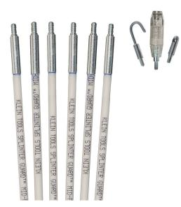
This specialty set of fish rods is the perfect solution for low-light applications. In addition to the six 5-foot glow rods, this set also includes an illuminated LED, a hook and a bullet nose tip making it a great option for telecom and datacom installations. The protective Splinter Guard™ coating on these fish rods guard your hands against fiberglass splinters. These mid-flex, 3/16-lnch rods can connect together easily up to a full 30-foot allowing wire to be pulled across long distances.
