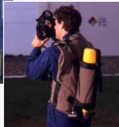
Lightweight, hoop-wrapped, 30-minute cylinder is positioned for ideal weight distribution and easier valve access.
