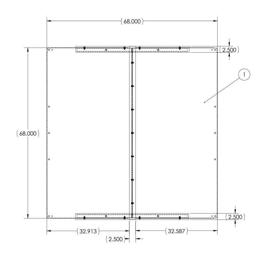
2.5 IN OF SPACE TO AVOID DRILLING IN MIDDLE AND TOP & BOTTOM EDGE
