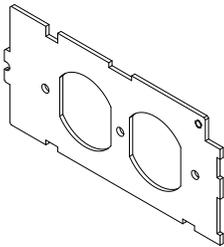
**Duplex Device Plate** - Accepts standard 15 Amp & 20 Amp Duplex Receptacles.
