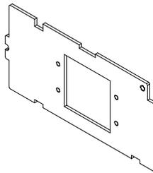
**MAAP Device Plate** - Accepts two (2) Legrand AVIP or Extron® Electronics MAAP Series Devices (sold separately)
