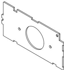
**1.39" Single Device Plate** - Receptacle opening 1 3/8" (35mm)
