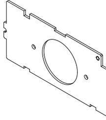
**1.59" Single Device Plate** - Receptacle opening 1 9/16" (40mm)
