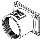
**2" Conduit Transition Hub** - Trade size 2" die cast zinc conduit fitting allows for 2" conduit to transition into a shallow box design. Includes: die cast fitting, gasket, and mounting screws.
