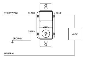
Three-way wiring diagram: Lights will turn OFF automatically when sensor that detected motion last, times out.
