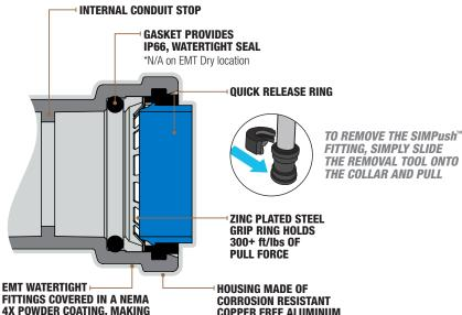
**4X POWDER COATING, MAKING IT READY FOR DIRECT BURIAL** AND CORROSION RESISTANT **\*N/A ON EMT DRY LOCATION**
