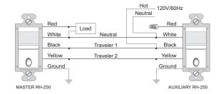
For single pole applications, cap off the yellow wire. Up to four multi-location sensors may be connected together. For details on connecting RH-253s for multi-location control, see the RH-253 cutsheet.
