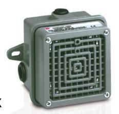
Model 350WB Vibratone® horn produces sound by the electro-mechanical vibration of a stainless steel diaphragm. The horn mechanism with diaphragm is attached to the grille. Indoor or outdoor use is made possible by the water- and dust-tight back box.
