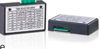
Model UTM is a microcontroller-based tone generator capable of producing 32 different tones. Model UTM is the key component of a SelecTone® System or a single SelecTone device. Tone selection is made by setting five DIP switches.
