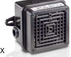
Model 350WBX Vibratone® horn produces sound by electro-mechanical vibration of a stainless steel diaphragm. The horn mechanism with diaphragm is attached to the grille. The water- and dust-tight back box is ideal for indoor or outdoor use
