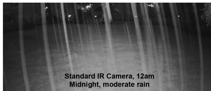
IR reflected off raindrops, obscuring view
