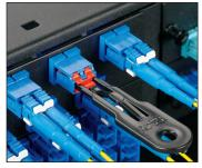
Insert the removal tool, which attaches to the blockout device
