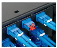
Snap the blockout device into the LC Duplex Adapter
