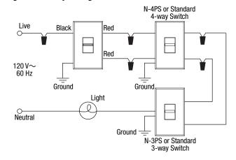
**Note:** Only one dimmer per 3-way circuit. Position of N-603P, N-1003P, N-1503P, N-2003P and 3-Way switch may be reversed in wiring diagram. 4-way switches must be wired between N-603P, N-1003P, N-1503P, N-2003P and 3-way switch.
