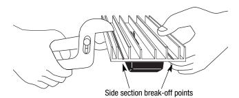
**Note:** When removing side sections, remove only inner side sections. **Do not** remove side sections on outer ends of the gang.
