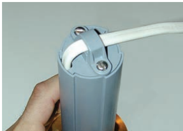
5. Secure wire clamp on bottom of tube.
