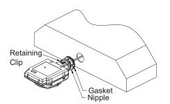
The sensor should be positioned so that heat radiating from the fixture does not affect its performance.
