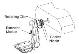
The EM1 Extender Module positions the sensor below the fixture.
