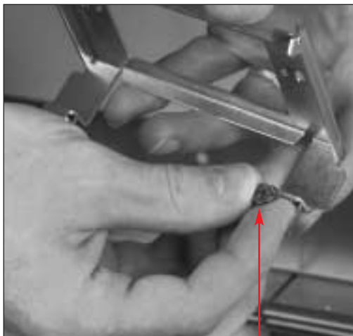
A #10-32 Ground Screw is provided on all Device Brackets.
