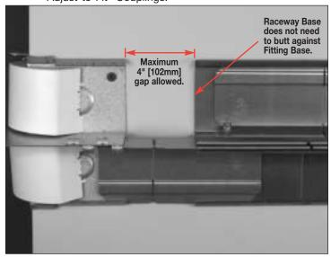
**Step 4.** Install Raceway Covers as shown. Position raceway cover section against cover stop and snap into place.
