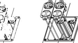
B. Mount the device in box by sandwiching the device to the box with the intermediate sub-plate using provided #6-32 x 3/4" pan head mounting screws. Note: Orient the Sub-plate to say "THIS SIDE UP". For the two port, attach the device to the box by screwing the strap directly to the box using provided #6-32 x 3/4" pan head mounting screws.
