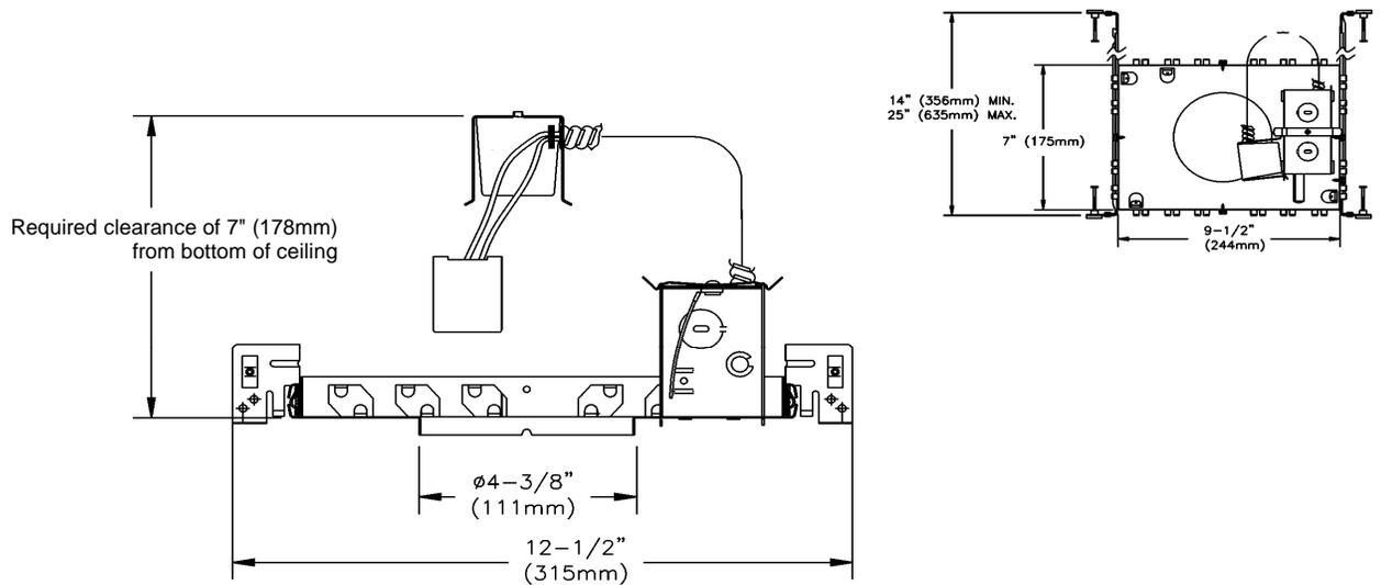
Complete fixture consists of Reflector Trim & Frame-in Kit. Select each separately.
