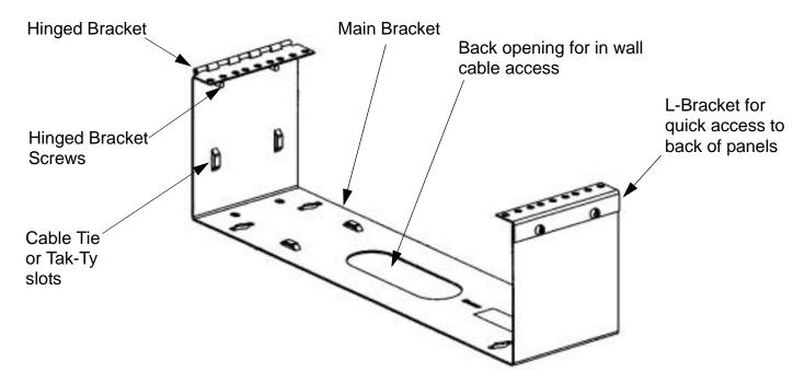
NOTE: WBHE models are packaged without hinges or L-brackets installed. Mount hinges and L-brackets on the outside of the Main Bracket as shown, using the supplied #12-24 screws and pem nuts. Make certain the pem nuts are facing the back of the Main Bracket.
