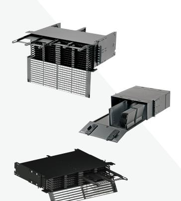
**Enclosures/Panels** – Drawers slide out into locked positions for easy MACs, and house cassettes and FAPs, trunks, connectors, and patch cords. Available in 1-RU, 2-RU, and 4-RU, supporting 144 fibers per rack unit, and can be reconfigured to accept 6-port or 12-port, cassettes or adapter panels.
