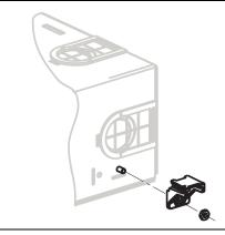
Attach strain relief clip with the #10-32 screw and nut provided.
