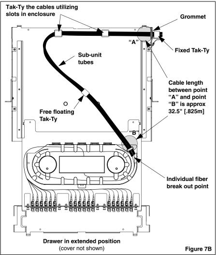
Route fiber through cable entry grommet as shown. Use enough cable length to ensure one complete loop of individual fibers around FOSM slack spools.
