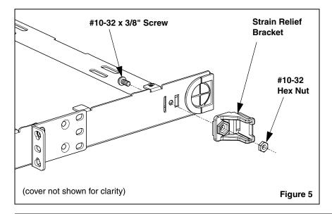
Install the strain relief bracket near where the cable will enter the enclosure. Secure with #10-32 x 3/8" screw and #10-32 hex nut.
