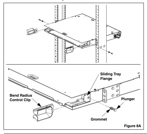
Install plunger into grommet, but do not fully seat. Slide bend radius control clip over the sliding tray flange as shown.
