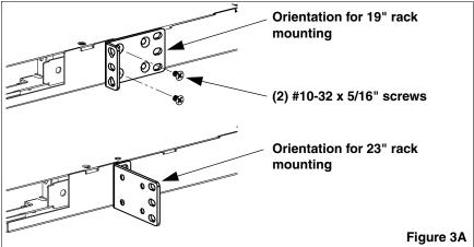
Determine the proper orientation for the mounting brackets according to rack size being used.
