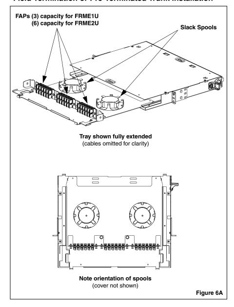
Slack Spools may be mounted with adhesive backing only or securing with #10-32 hex nuts.
