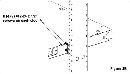
Place enclosure mounting brackets at desired position on the rack. Mount the enclosure to the rack using (4)  $\#12-24 \times 1/2$ " screws.
