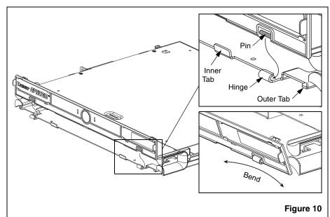
Install the front door as follows. Install the rear door in a similar manner.
