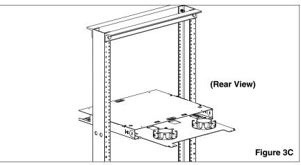
Enclosure is accessible from the rear for mounting of slack spools, Fiber Optic Splice Modules (FOSMs) and other equipment.
