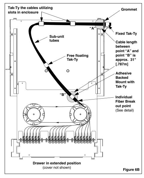
Route fiber through cable entry grommet as shown. Use enough cable length to ensure one complete loop of individual fibers around slack spools. Leave enough jacketed slack so when the drawer is fully extended the cables are not put under tension. DO NOT use so much slack that the drawer cannot be returned to its home position. (See Figure 6C)
