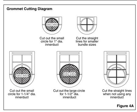
After the enclosure is mounted to the rack, determine the size of the innerduct (if any) that will be used to bring the cable into the enclosure. Prepare grommet according to the proper cutting diagram to the left.
