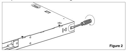
Determine where the cable will enter the enclosure. Carefully remove the knock-out so as not to damage the surrounding sheet metal. DO NOT install the grommet at this stage. Grommet will be installed after the enclosure is mounted to the rack.
