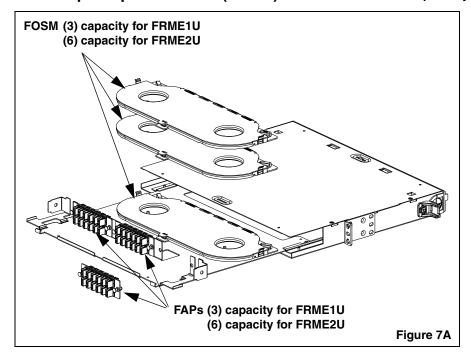
Place first FOSM over #10-32 studs on sliding tray and secure with #10-32 hex nuts. Remaining FOSMs are stacked on top of each other and snap in place.
