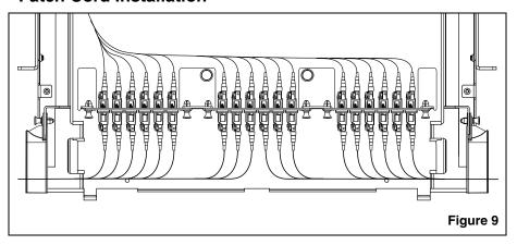
Install patch cords into FAPs routing through bend radius control clips and maintaining proper patch cord bend radius.
