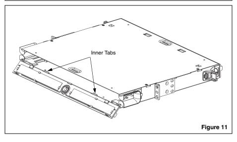
The final door position should be on the outside of the inner tabs.
