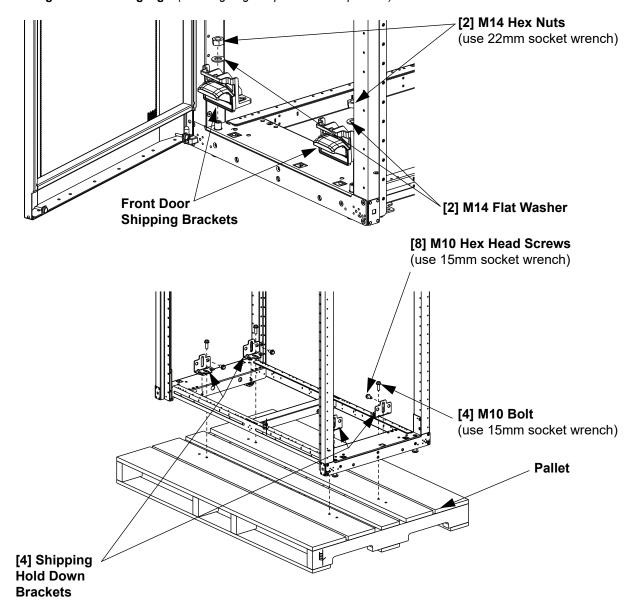
Note: Doors, Side panels, and other components are removed for clarity.
