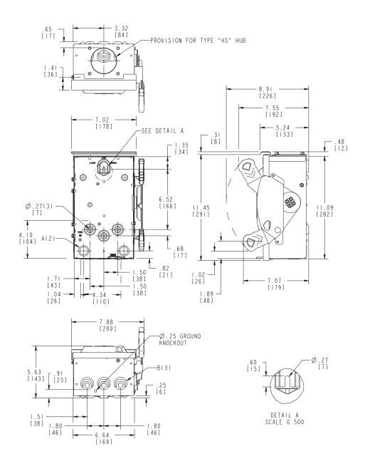
No knockouts in enclosures. Dimensions shown in inches and millimeters ( ). Dimension shown accurate to  $\pm \frac{1}{8}$  inch.
