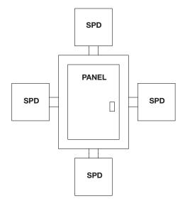
6. Using a hole saw (or knockout device), cut a hole in the SPD enclosure at the entrance location. The upper edge of the hole must not exceed 1.3" from the mountable bottom of the SPD enclosure (see figure at right). Duct hole location must be centered to the side chosen. Remove any dust, residue and/or burrs from the SPD housing after making the knockout.
