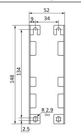
Fig. 25-7 Wall/panel mounting, side view
