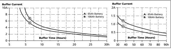
The battery capacity is usually specified in amp-hours (Ah) for a 20h discharging event. The battery discharge is nonlinear (due to the battery chemistry). The higher the discharging current, the lower the appropriable battery capacity. The magnitude of the reduction depends on the discharging current as well as on the type of battery. High current battery types can have up to 50% longer buffer times compared to regular batteries when batteries will be discharged in less than 1 hour.
