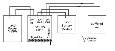
Fig. 26-3 Wiring example for inhibit input
