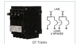
These space saver triplex breakers provide a 2-pole common trip breaker for 120/240V AC circuits and two single poles for 120V AC circuits. Triplex require two panel spaces. HACR rated.
