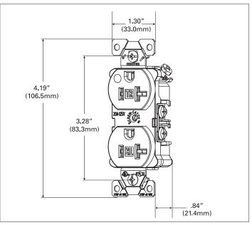
Figure 4. TR8300 Line art with dimensions
