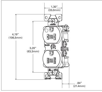
Figure 3. TR8200 Line art with dimensions
