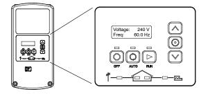
The RDC2 controller provides integrated control for the generator set, Kohler® Model RXT transfer switch, programmable interface module (PIM), and load shed kit.
