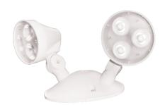
The RMSM series of commercial thermoplastic PAR18/MR16 remotes provides the perfect balance of value and performance. The heads are fully adjustable and both tilt and swivel are lockable. The standard canopy is designed to mount directly to typical electrical junction boxes. Available in 6 V, 12 V and 24 V models, utilizing either LED, tungsten or quartz halogen lamps.
