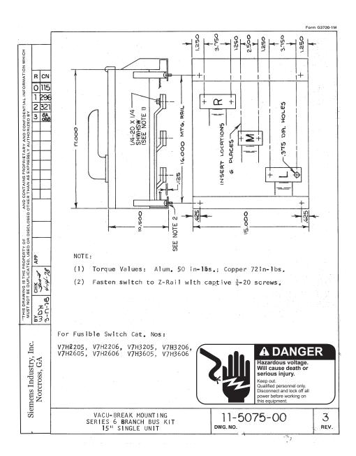
FOR USE WITH 15.0" SINGLE UNITS ON SERIES 5 OR 6 DISTRIBUTION SECTIONS, CDP-5, CDP-6, VB-5, VB-6, FCI, FCII, SB1, SB2 & SB3.
