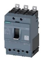
circuit breaker 3VA4 UL frame 125 breaking capacity class H 65kA @ 480 V 3-pole, line protection TM210, FTFM, In=100A overload protection Ir=100A fixed short-circuit protection Ii=10 x In clamp connection
