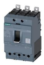
circuit breaker 3VA4 UL frame 125 breaking capacity class H 65kA @ 480 V 3-pole, line protection TM210, FTFM, In=25A overload protection Ir=25A fixed short-circuit protection li=12 x In clamp connection
