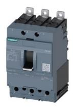
circuit breaker 3VA4 UL frame 125 breaking capacity class H 65kA @ 480 V 3-pole, line protection TM210, FTFM, In=90A overload protection Ir=90A fixed short-circuit protection li=10 x In clamp connection
