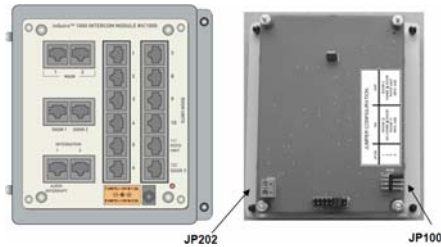
Figure 11 - Install Intercom Module into Enclosure
