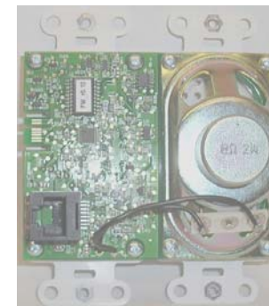
Figure 6 - Plug Room Cable into Room Unit
