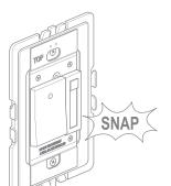
NOTE – If you need to remove dimmer after snapping into frame, first remove frame from wall box to access the four locking tabs on the back of the dimmer. Insert a flat screwdriver to depress tabs as you apply pressure to push dimmer out.
