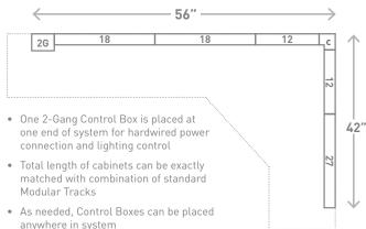
**Sample Installation:** Length of cabinets is greater than combined length of standard Modular Tracks
