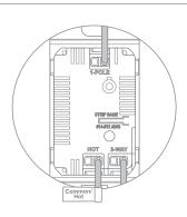
**NOTE** - In a 3-Way installation, use one dimmer and one switch. Do NOT use two dimmers.
