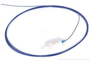
Fiber patch cords provide connections from the work area to the wall outlet, or from active equipment to the patch panel. Cords are available as duplex or simplex 62.5/125, 50/125 MM or SM fibers. We offer ST-style, SC, MT-RJ or LC connectors. 1.8mm/2.0mm jacket diameter takes up less space for greater patch cord density. 1.8mm/2.0mm jacket diameter takes up less space for greater patch cord density. All patch cords are factory polished and 100% optically tested for superior performance.
