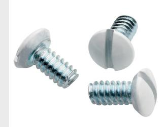
Oval head milled slot 1/2" long, 6x32 thread. Standard size for duplex receptacles and toggle switch wall plates. White.
