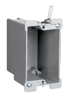
Durable, impact-resistant thermoplastic box complemented by innovative extras that cut installation time. Single Gang, Old Work Switch and Outlet Box with Swing-Bracket for mounting. Adjusts from 1 1/4" down to 1/8". Two Auto/Clamps on Each End. 100 pack.
