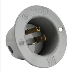
Straight Blade 2pole 3wire 20amp 125volt Flanged Inlet
