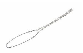
Standard-duty, Closed mesh, Single eye grips. Cable diameter - 0.620-0.740", Bale length - 8", Mesh length - 11", Break strength - 960 lbs.
