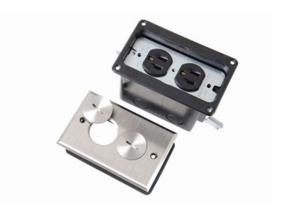
Tamper-Resistant Floor Box Assembly. #8 duplex opening. Two threaded screw plug, Includes 3232 15 amp, 125 volt tamper-resistant receptacle. Nickel.
